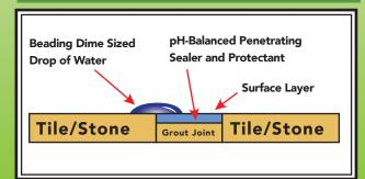
**NOTE:** If the water drop is smudged into the surface layer of the grout and stone and then wiped dry, it may appear that the water drop has penetrated the grout and stone surface layer. In reality, the grout and stone has only been affected on the surface layer and has only obtained "surface layer wetness."
